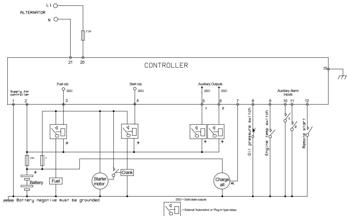
Terminals suitable for 22-16 awg (0.6mm<sup>2</sup>-1.3mm<sup>2</sup>) field wiring
