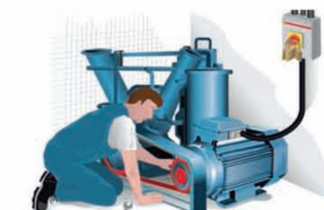
Safety switches protect the operator from unexpected start-up
